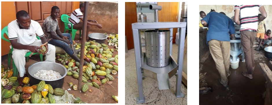
Figure 2: Demonstration of removing cocoa bean pulp from pods and extraction of juice using stainless juice extractor
