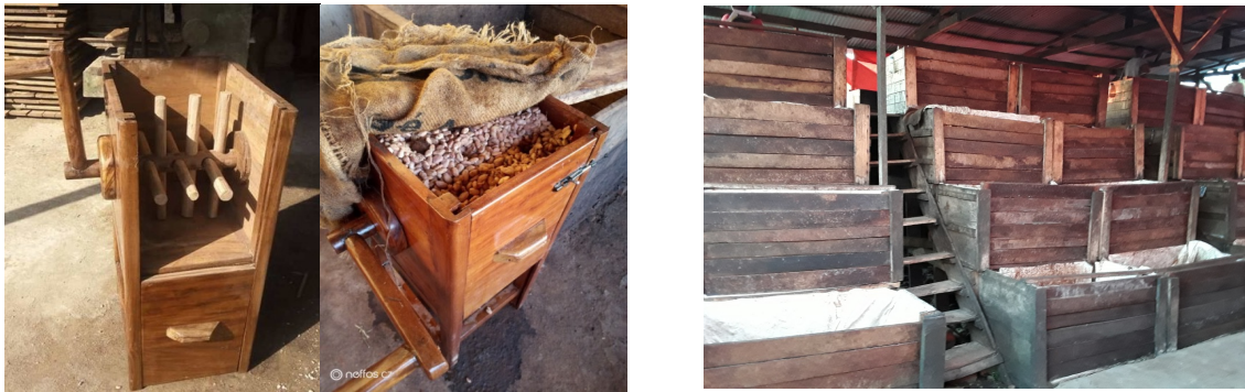
Figure 1: Left hand is the single fermentation box showing the inside design and a filled box with cocoa; on the right hand is the storeyed fermentation box with steps for climbing while filling first box
