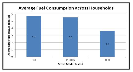
Figure Graph of average daily fuel consumption against stove model tested during KPT
