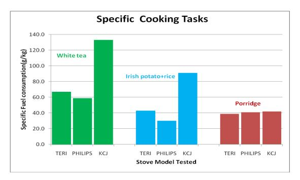
Graph of Specific fuel consumption against stove model tested during CCT
